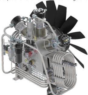
The bearings of the crankshaft have rollers, extremely robust and made in Europe which guarantee a long life of the compressor. An oil pump provides a constant lubrication of the inner workings of the block with oil cleaned of impurities by a filter and by a magnet which catches any metals present in the lubricating oil.
